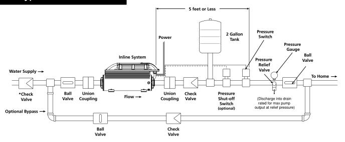
\*NOTICE: If system plumbing does not have a backflow prevention device, a check valve is required on the incoming water supply line.
