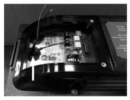
Attach the wires to terminal labeled "Shut-off Sensor". The red wire goes on the outside left terminal and the black wire goes to the inside right terminal. Use 4 in/lbs (0.45 N-m) of torque.
