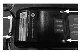
6. Loosen the small strain relief.
