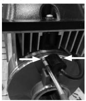
4. Route the thermostat wire across the top of the pump, running it between the
