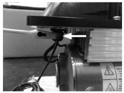
Route the thermostat cable through the small strain relief with the pressure sensor wire.
