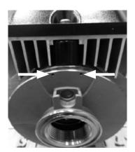
3. Use the two supplied lock washers and screws to affix the thermostat to the pump using 4 in/lbs (0.45 N-m) of torque.
