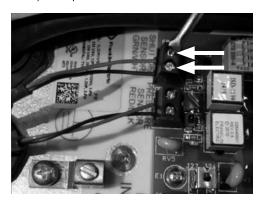
9. Tighten the small strain relief with 50 in/lbs. (5.65 N-m) of torque.
