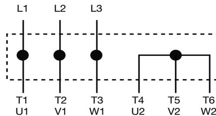
Each motor lead is numbered with two markers, one near each end. To reverse rotation; interchange any two line connections.
