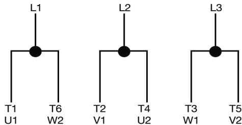
WYE-DELTA starters connect the motor as shown below during starting, then change to the running connection shown at the left.
